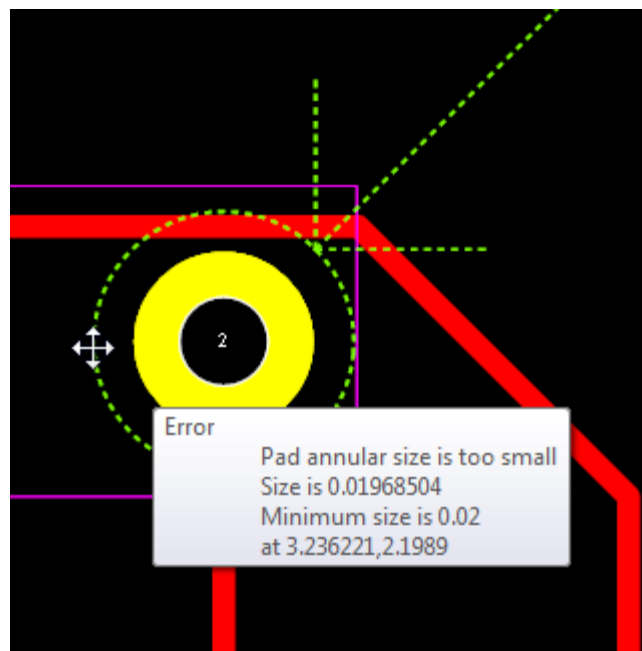
Pad annular ring too small - marked with green circle (and arrow if error selected)
